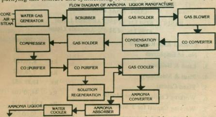
sence of a suitable catalyst. Water gas is first produced by passing steam on coke. The nitrogen required for ammonia synthesis is usually furnished by adding a sufficient quantity of the products of combustion from the blasting step to the gas stream. Water gas is further mixed with steam and passed through a catalyst in converter to convert CO to CO<sub>2</sub>. Converted
